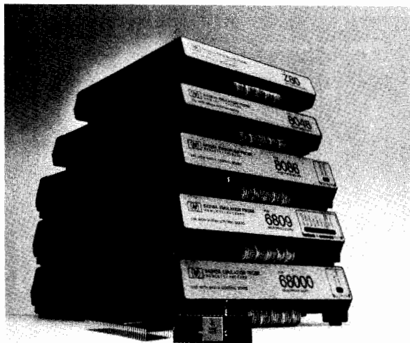
Figure 4. Emulation subsystems are available for a variety of 8-bit and 16-bit microprocessors. Emulation pods are shown for some of the supported processors.
