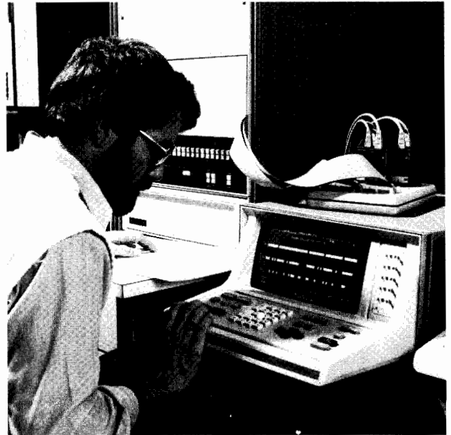
Figure 9. The logic state analyzer is an excellent troubleshooting tool for hybrid logic circuits, and is frequently used to supplement the development system for digital measurements.
