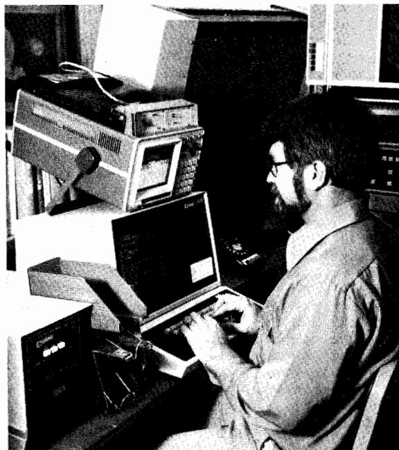
Model 1640B Serial Data Analyzer monitors or simulates serial data transmissions in computer networks which use the RS-232-C (V.24) interface.
