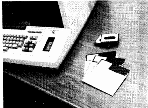
Figure 13. Software for the 64000 Logic Development System is available on flexible discs or tape cartridges.
